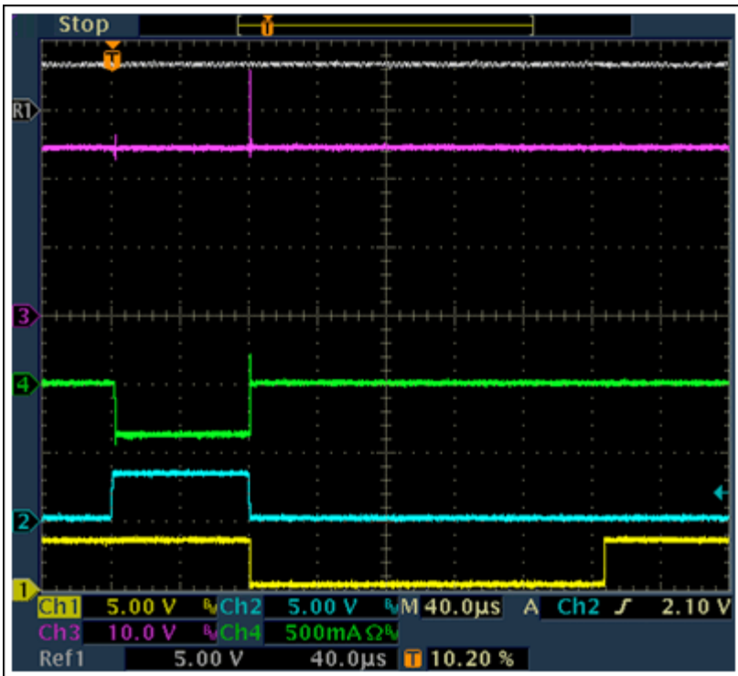
Figure 1. Valid wake-up detection in push-pull mode (R1 = TXEN, CH3 = C/Q, CH4 = current out of C/Q, CH2 = TXC = TXQ, CH1 = /WU).
