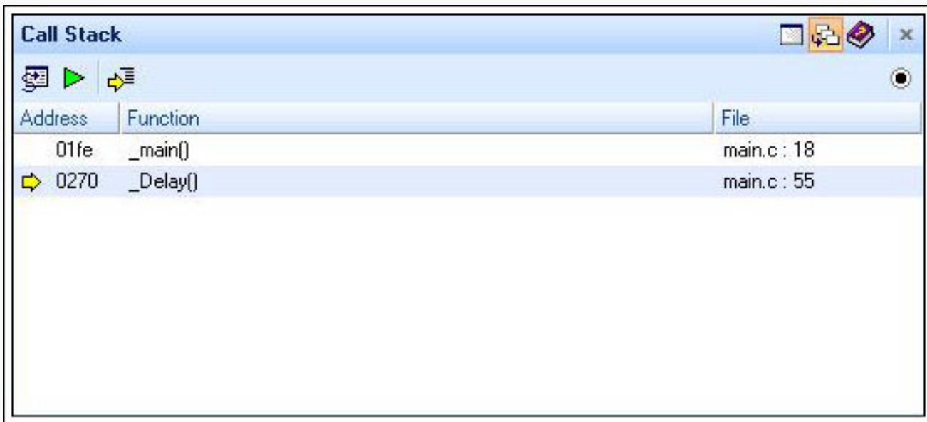
Figure 10. Call Stack while running in the Delay() function.
