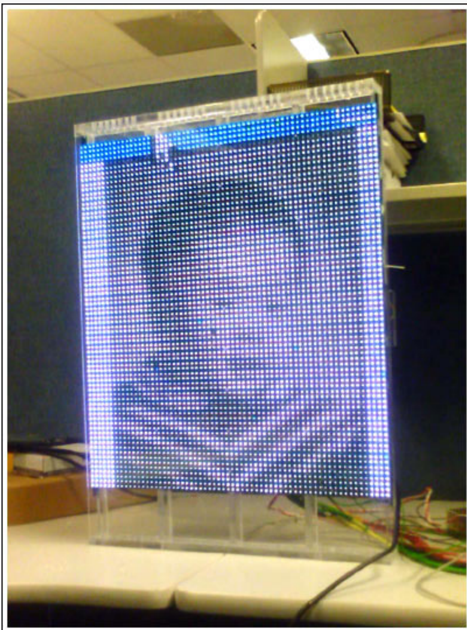
Figure 10. An acrylic frame that houses up to 10 LED PCBs.
