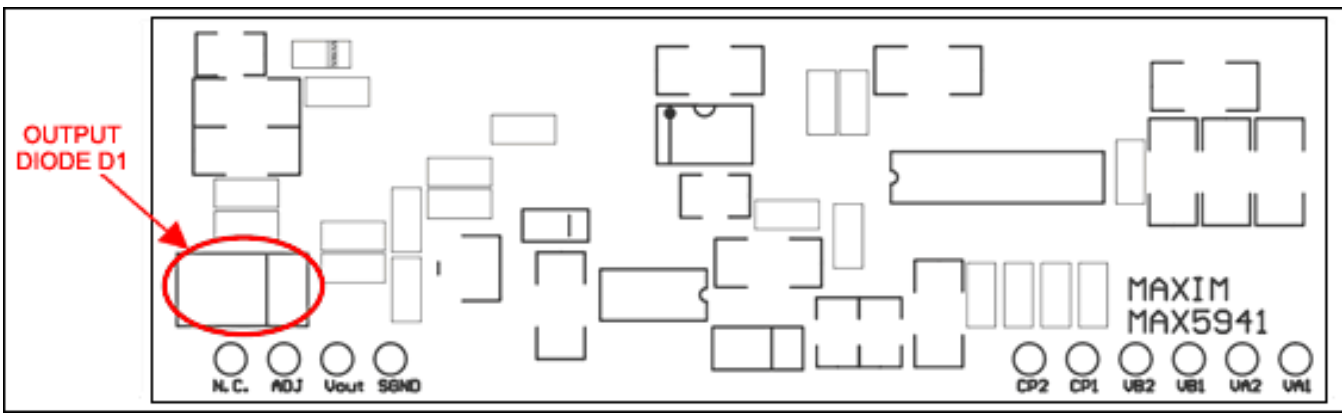
Figure 7. The location of the internal diode D1 on the MAX5941B PD module.
