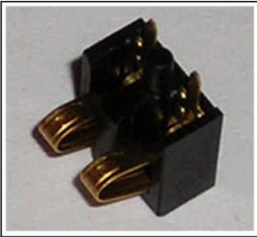
Figure 9. Contact B, Suyin 060121MR Series. Part number as shown: 060121MR002G_00ZU (_ = place holder for plating specification). Description: 3.60mm Pitch 2 Pin Battery Connector Spring DIP Type. Note: The product is pictured "upside down," i.e., the pins and the center-post are designed for through-mounting on a circuit board.
