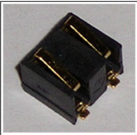
Figure 10. Contact C, Suyin 425122MA Series. Part number as shown: 425122MA002G_00Z_ (_ = place holders for plating specification and tube or reel). Description: 4.25mm Pitch 2 Pin Battery Connector SMT Type.
