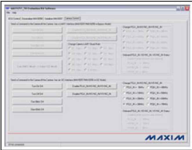
Figure 7. The upper portion of the Camera Control page is grayed out, indicating that I 2 C mode is enabled.
