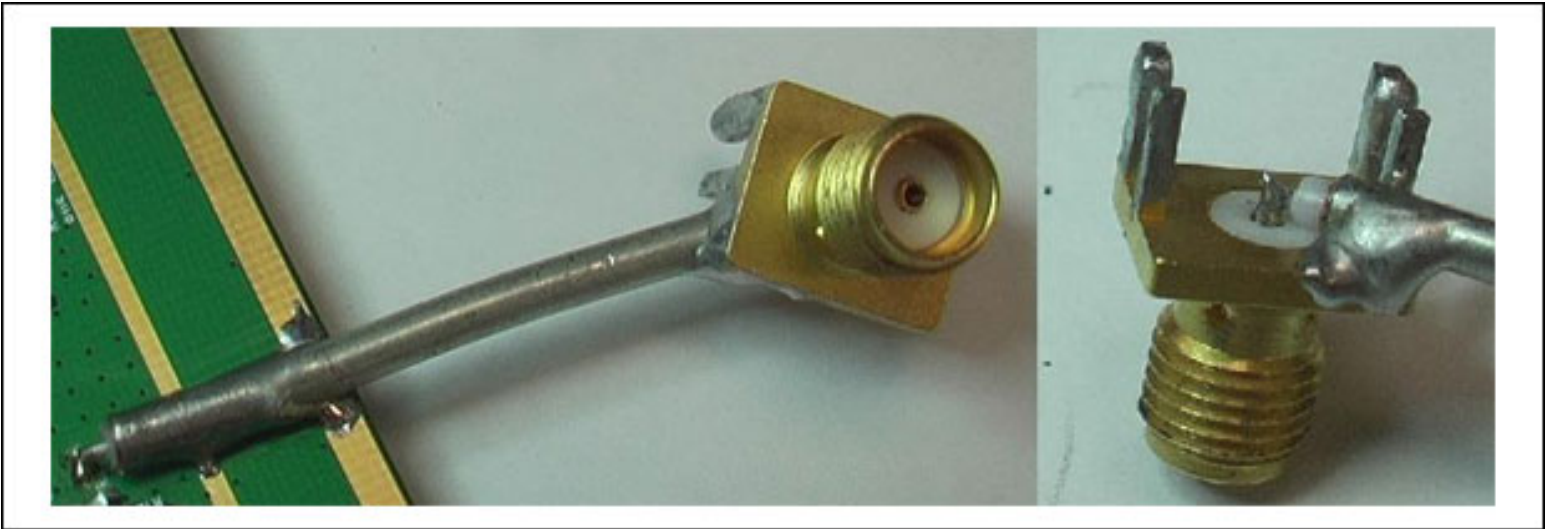
Figure 2a. Handmade microcoaxial cable—good to approximately 2GHz to 3GHz.
