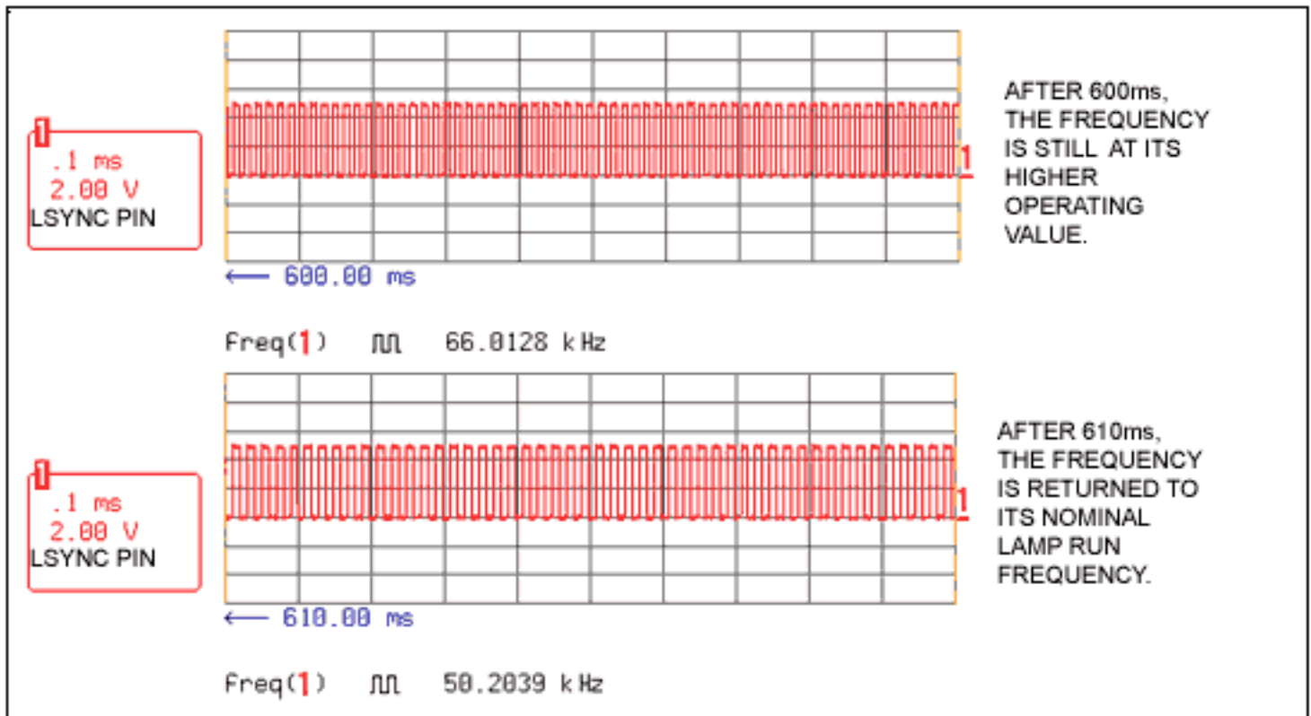
Figure 6. DS3881/DS3882 controllers return to nominal lamp run frequency.
