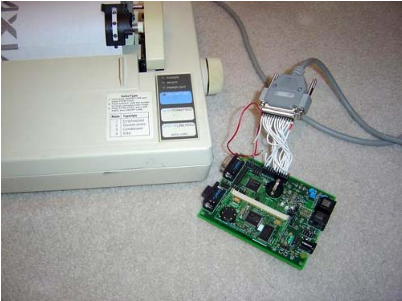
Figure 3. TINI400 socket board connected to the Epson printer.
