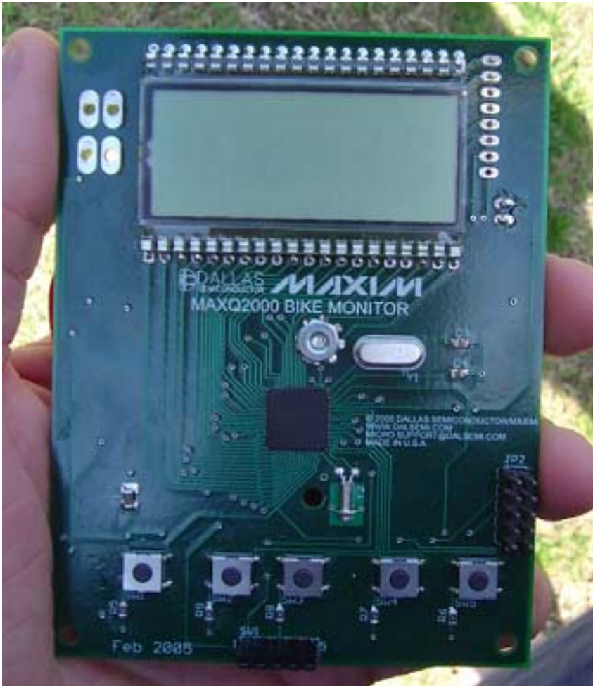
Figure 4. The bike monitor board. The backside has a 1-Wire can holder for the DS1923, a battery holder for three AA batteries, and connection pins to run to the DS2423 circuit.
