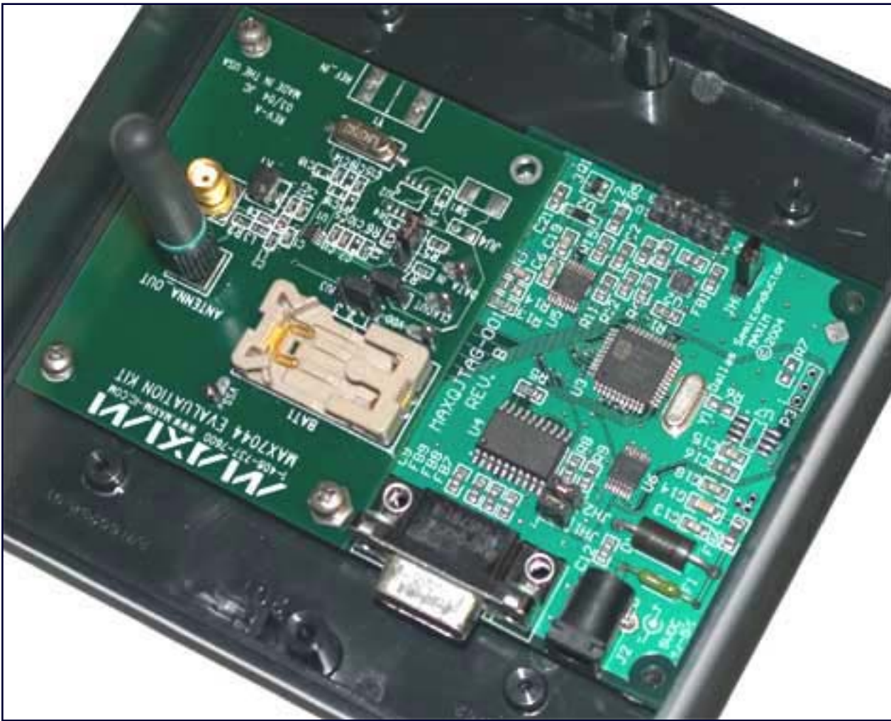
Figure 4. The key-fob transmitter uses two EV kits side by side.
