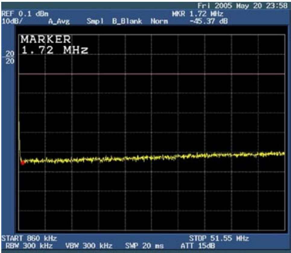
Figure 2. Return loss of 75Ω test load.
