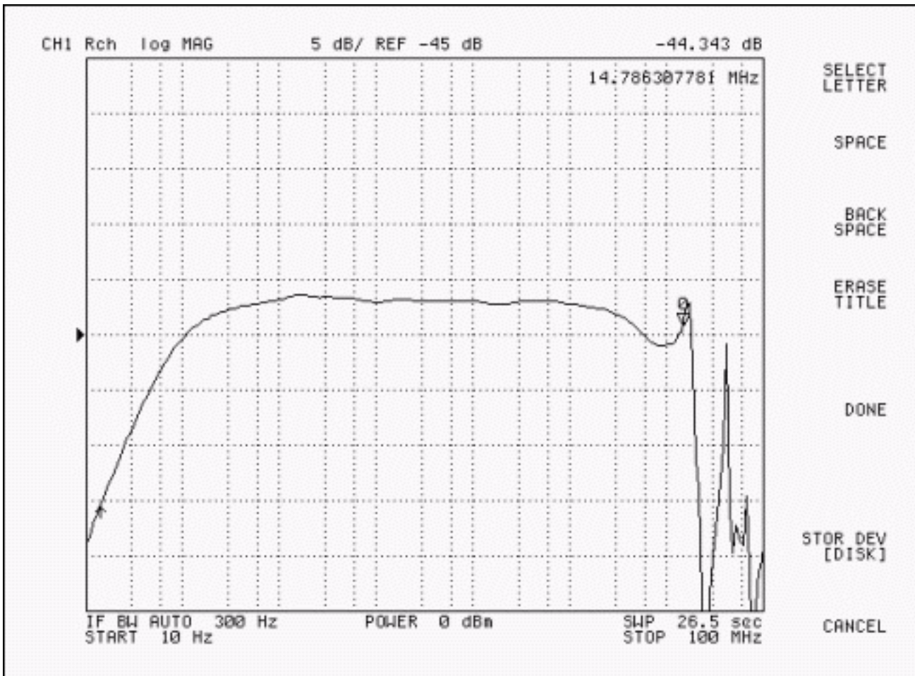
Figure 2. Frequency response of the PE-51687 transformer with a 22- \Omega resistor on the secondary.
