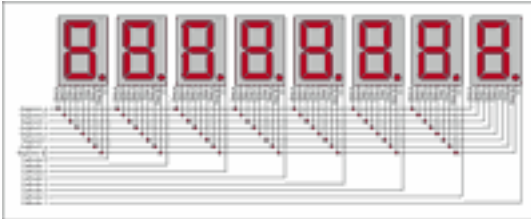
Figure 1. The MAX7219 and MAX7221 use standard connections - 16 pins to drive 8 digits.
