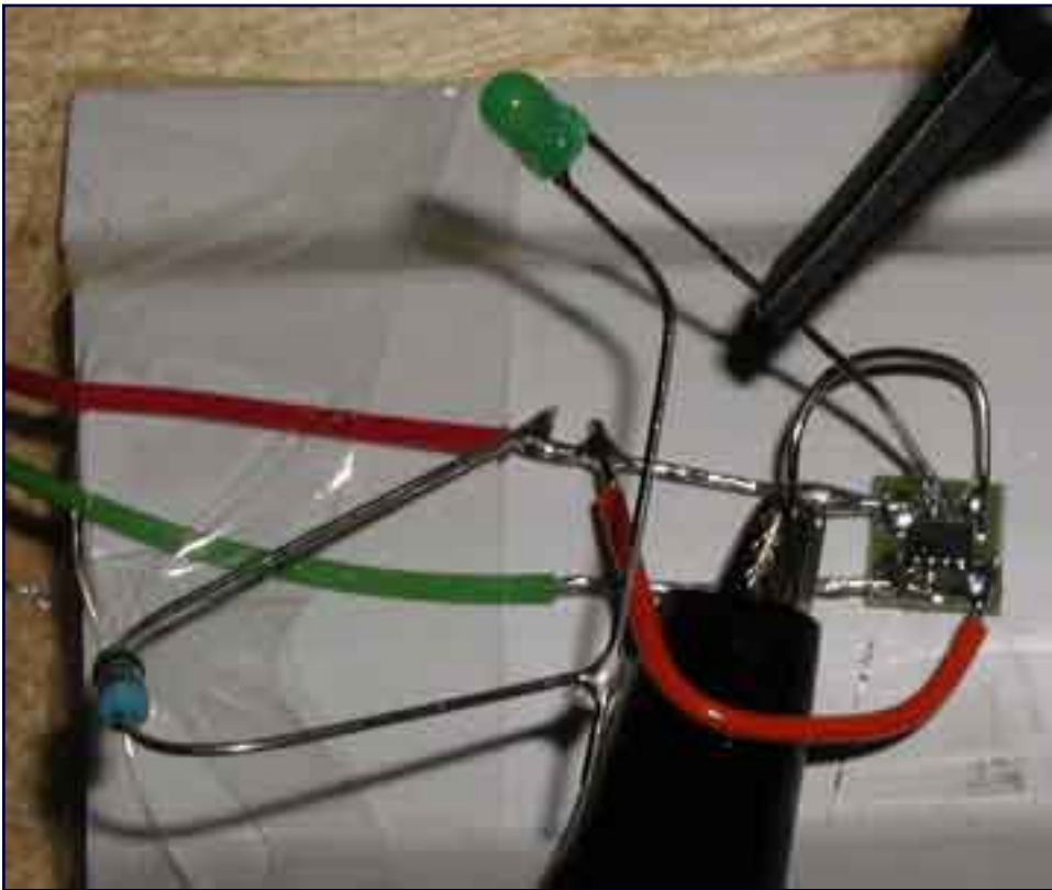
Figure 4. Picture of prototype blinking LED circuit.
