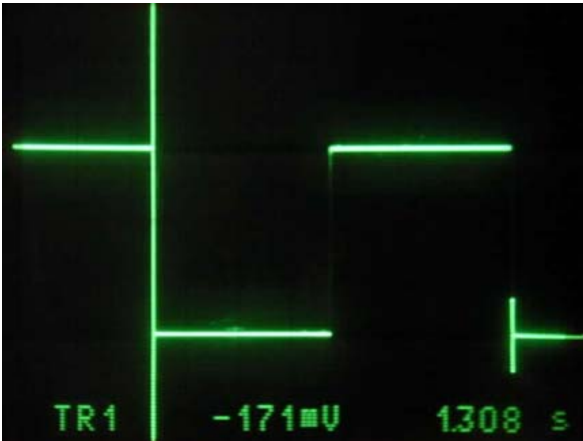
Figure 3. Comparator output; horizontal scale = 200mS/div, vertical scale = 500mV/div, supply voltage = 1.7V, amplitude = 1.7Vp-p, period = 1.308 seconds.
